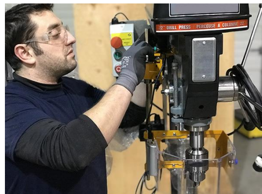
Installation of an interlock guard and motor starter station on a new drill press
