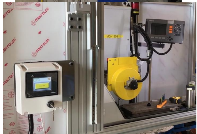
Surface grinder with pneumatic wheel to cover when the automatic gate door is opened. All controls are done through a touch screen & PLC programming
