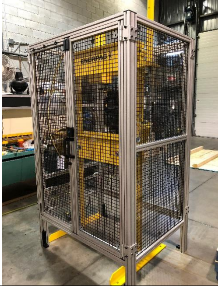
Hydraulic Insertion Press cage; interlocked doors with dual pressure system
