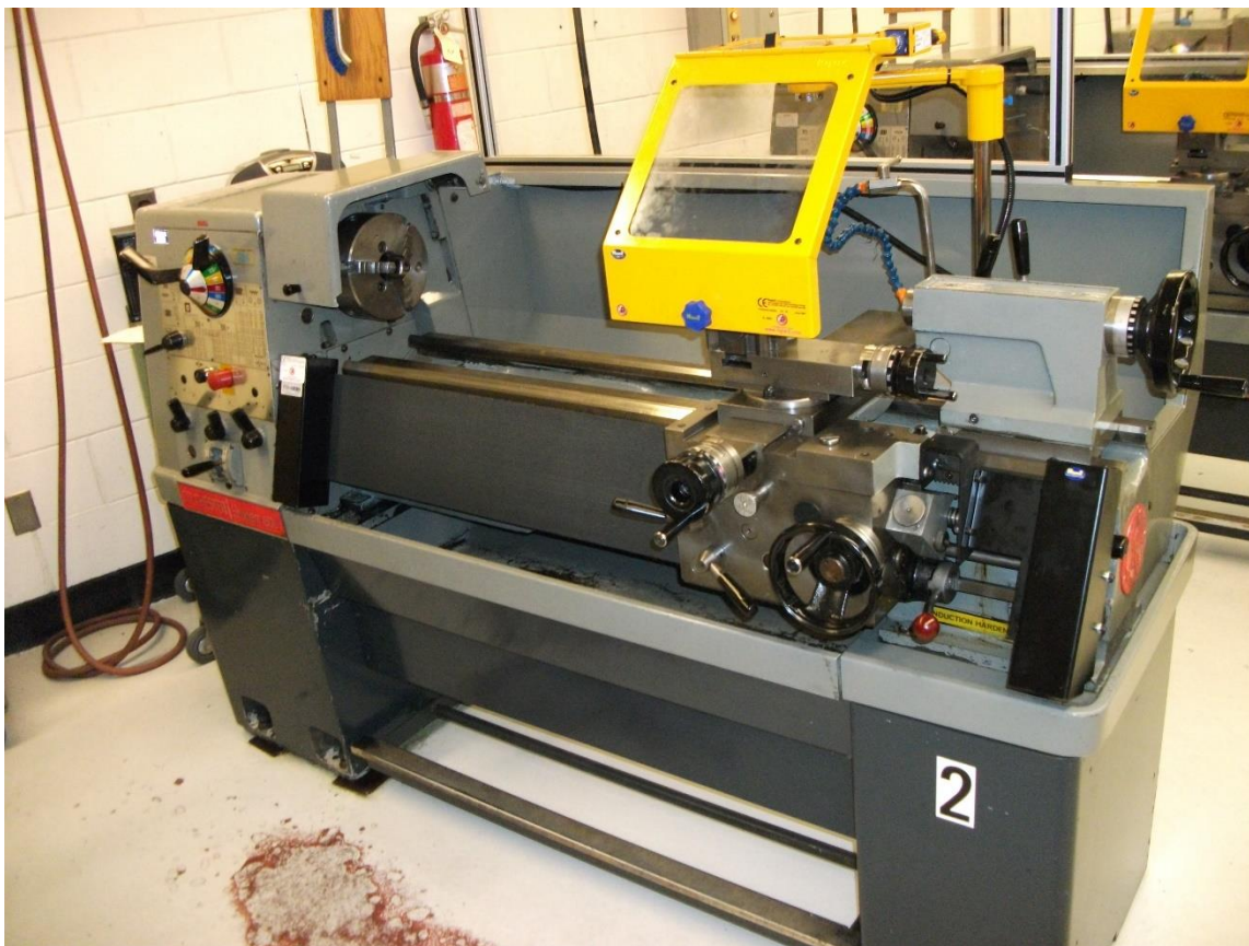
Figure 2 Lathe with AR lead screw guard installed.
