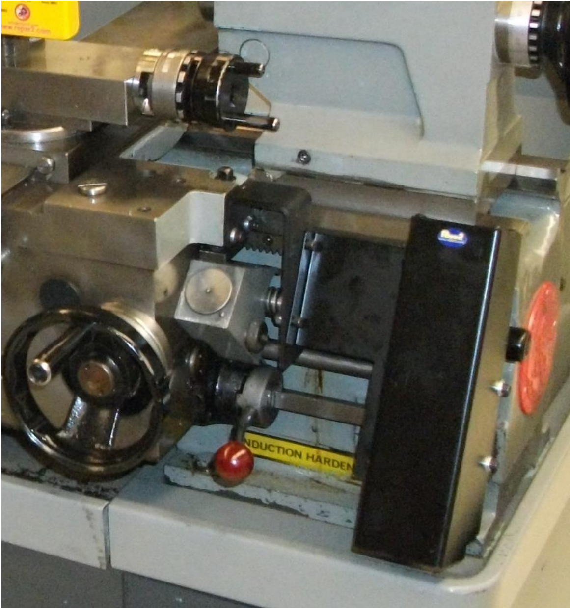
Figure 3 Detail of right-side AR and manufactured bracket made to go over threading dial
