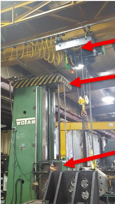
This is the **overhead gantry crane**. The crane is shown nearly in contact with the black-and-yellow striped section of the machine.
